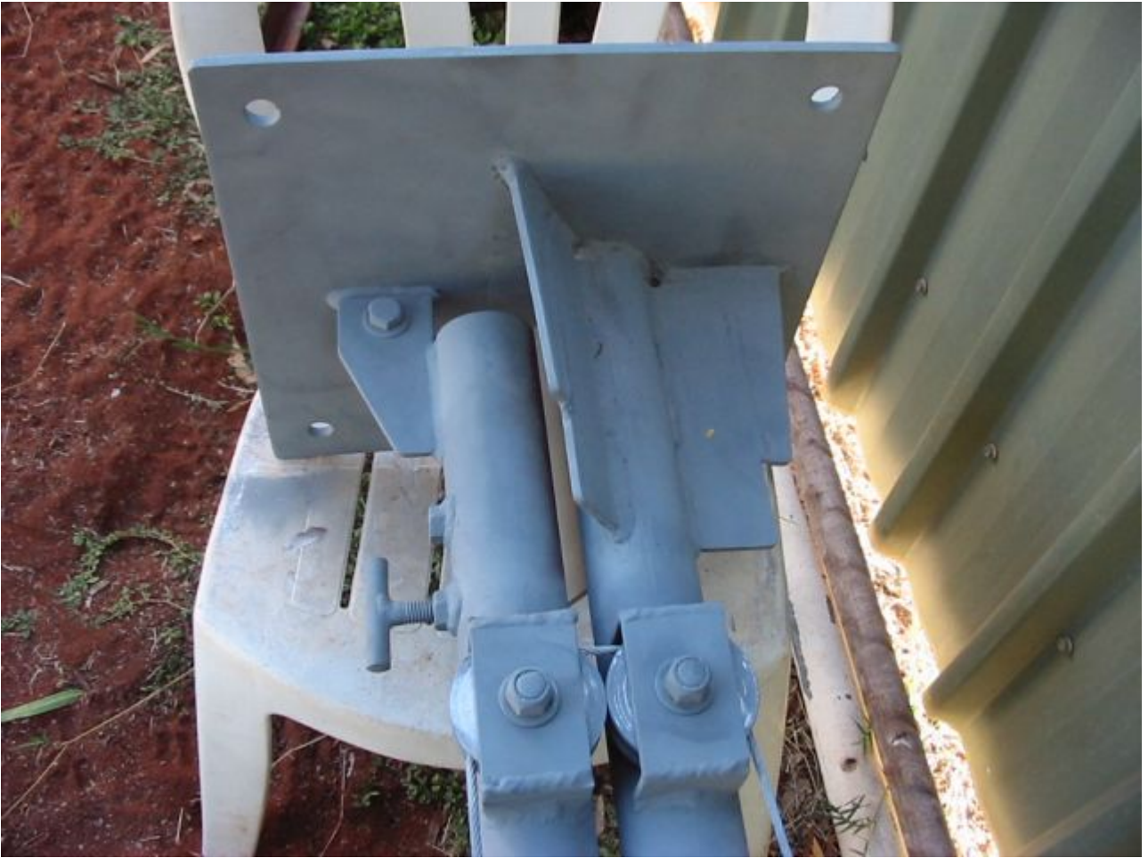
BOTTOM PULLEYS AND "THE BOLT". IN, TOWER TELESCOPES. OUT, TOWER TILTS OVER.
