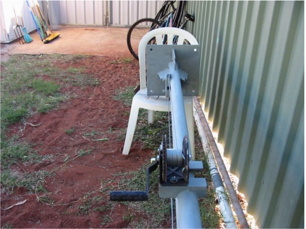
WINCH, PULLEYS AND BASE.
