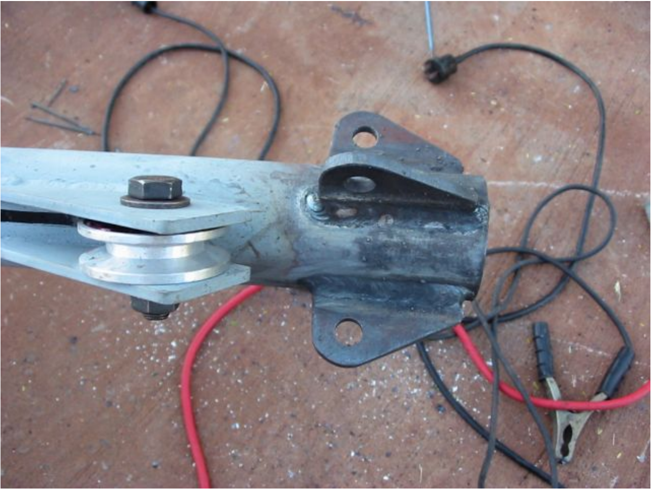
TOP PULLEY AND MIDDLE GUY WIRE POINTS
