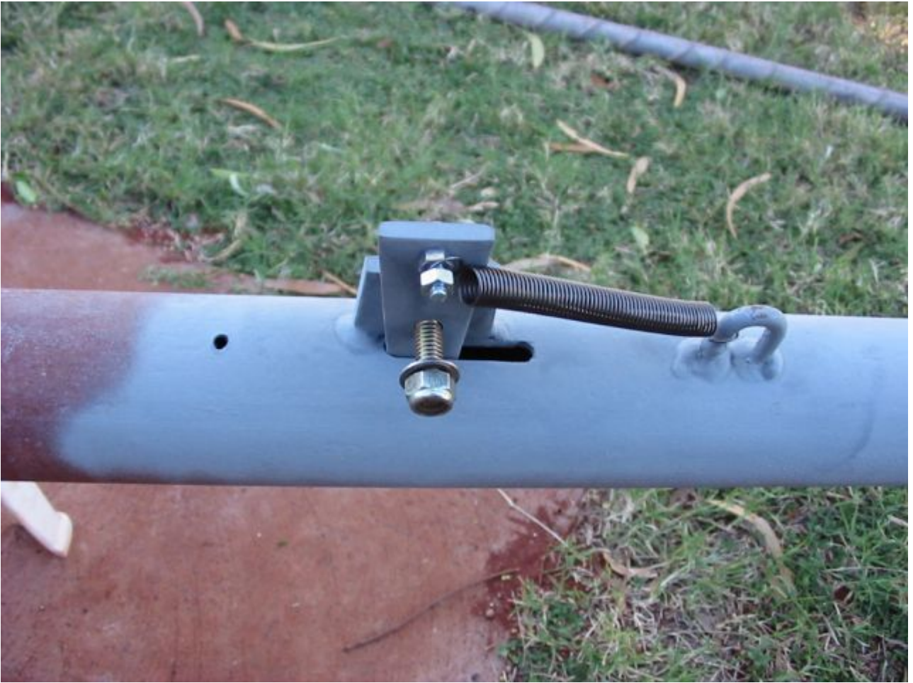
LOCKING PIN FOR LOCKING THE BOTTOM SECTION IN AT 12 METERS.
